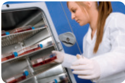
Sealed inner glass doors, standard in 170 L models, allows viewing access while maintaining sample integrity
