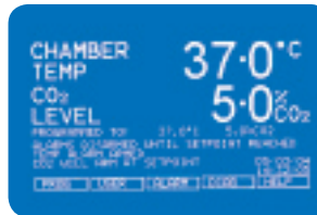
R Series LCD display, standard on 170 R and 48 R models
