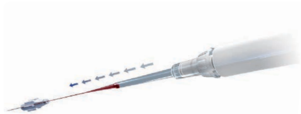
Rear filling of microinjection capillaries using Microloader
