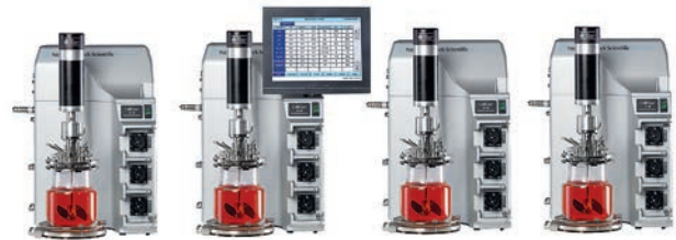
Up to four reactors can be controlled with a single Control Station.
