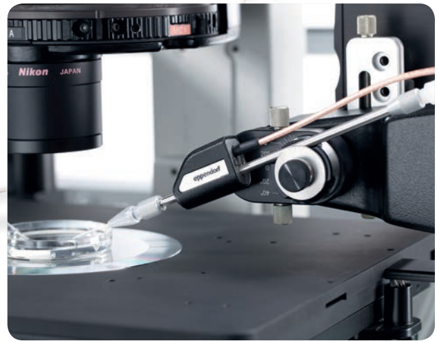
Eppendorf PiezoXpert actuator mounted onto the TransferMan NK 2
