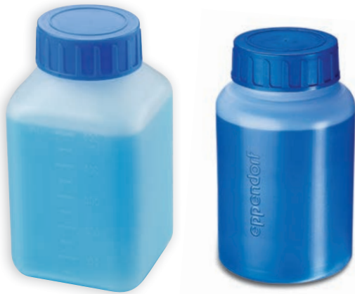
500 and 400 mL wide-mouth bottle for rotor A-4-81*1 (80 x 135 mm, polypropylene, centrifugation resistance up to 3,250 x g, autoclavable)
