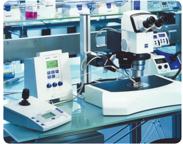
Workstation for microinjection into fish embryos: InjectMan NI 2, Zeiss SteREO Discovery.V12 and microinjector FemtoJet express
