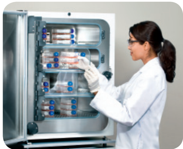
Split inner door option – improves uniformity and reduces gas consumption. 4- & 8-Split doors available on 170 L models. 2-Split doors available on 48 L models.
