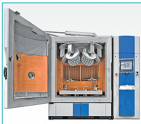
Photo courtesy of Leybold Optics. Syrus Pro 1510 LION Assisted Electron Beam Custom Ophthalmic Coater. Our engineers have worked closely with Leybold Optics of Germany to refine the performance of this large coating tool for the precise deposition of complex multi-layers for Image Enhancement coatings under the SpectraPlus brand.
