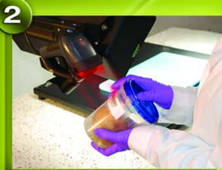
2 Sample log in validates the Case-Sample relationship avoiding mismatches (via keystroke or barcode).
