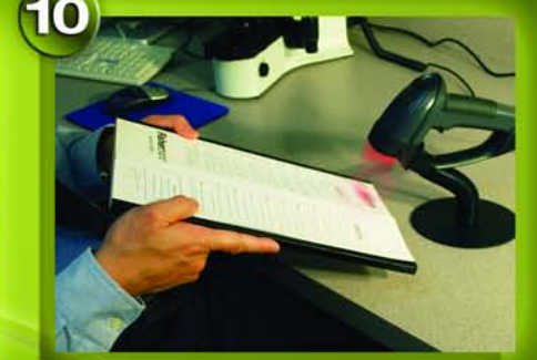
10 Slide index log in validates the Case-Sample relationship, avoiding mismatches (via keystroke or barcode).
