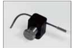
Perfusion Block This block is fixed on the metal plate by magnet. (locate block anywhere on the plate)
