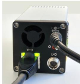
When there is communication between the camera and the computer, the left LED light will flash intermittently.
