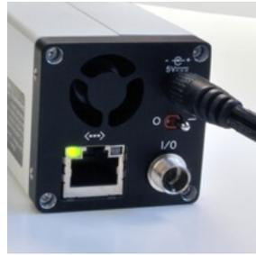
When the Ethernet cable is properly connected between the computer and the camera, the green LED light on the top right of the Ethernet port will be on.
