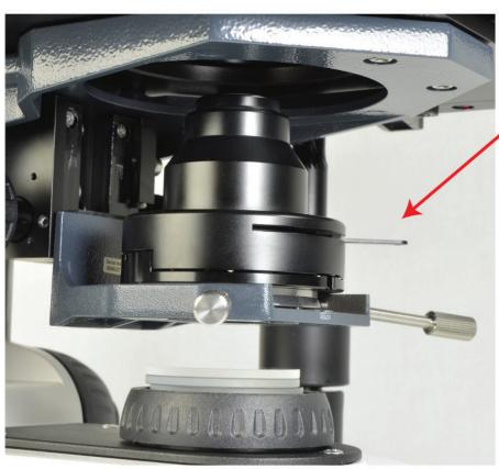
Open the Condenser Iris Diaphragm (under the stage) all the way open (to the largest number or all the way to the left).
