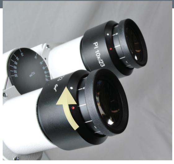
Rotate the front of the eyepiece until the "0" setting lines up with the white dot.
