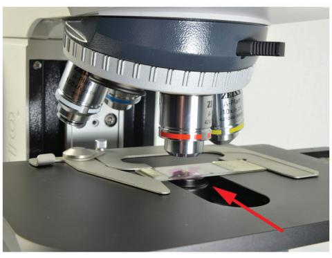
Raise the condenser until the top of the condenser almost touches the bottom of the slide.
