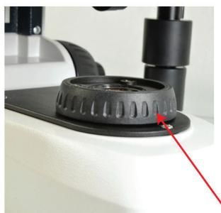
Open the Field Iris Diaphragm (in the front of the base) all the way open (typically turn all the way counterclockwise, you will see more light come out).
