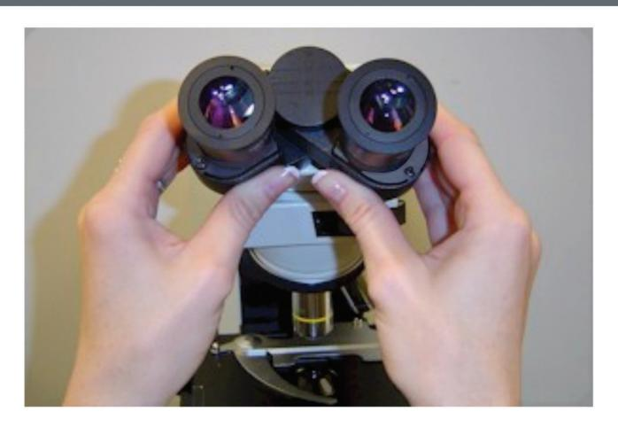
While looking through the eyepieces, adjust the interpupillary distance so that the microscope image can be seen with both eyes open. (This will take some practice!)
