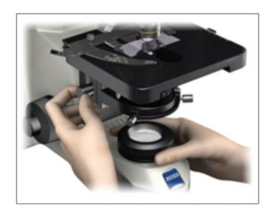
Look through the eyepieces and turn the condenser focus knob until the field diaphragm comes into sharp focus.
