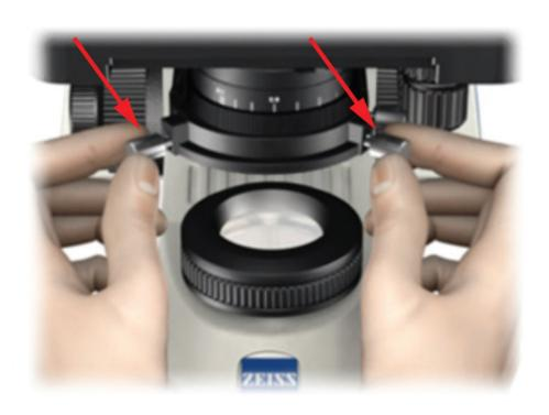
While looking through the eyepieces, use the condenser centering knobs to center the field diaphragm in the center of the field of view.
