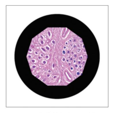
Keep opening the field diaphragm while adjusting the centration. Perfect centration is achieved when all of the outside "points" of the diaphragm equally touch the edge of the field of view.
