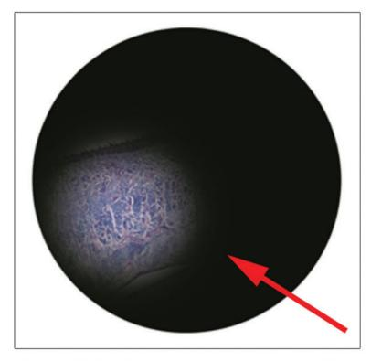
As the field diaphragm closes you will see the blurry, out-of-focus edges of the diaphragm move into the field of view.
