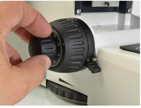
While looking through the eyepieces, use the (coaxial) coarse and fine focus knobs to bring the slide into focus.
