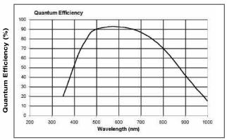
Quantum Efficiency at 575nm and -20° C9
