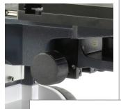
**Step 4:** Adjust the condenser focus knob until the edge of the field diaphragm comes into sharp focus.
