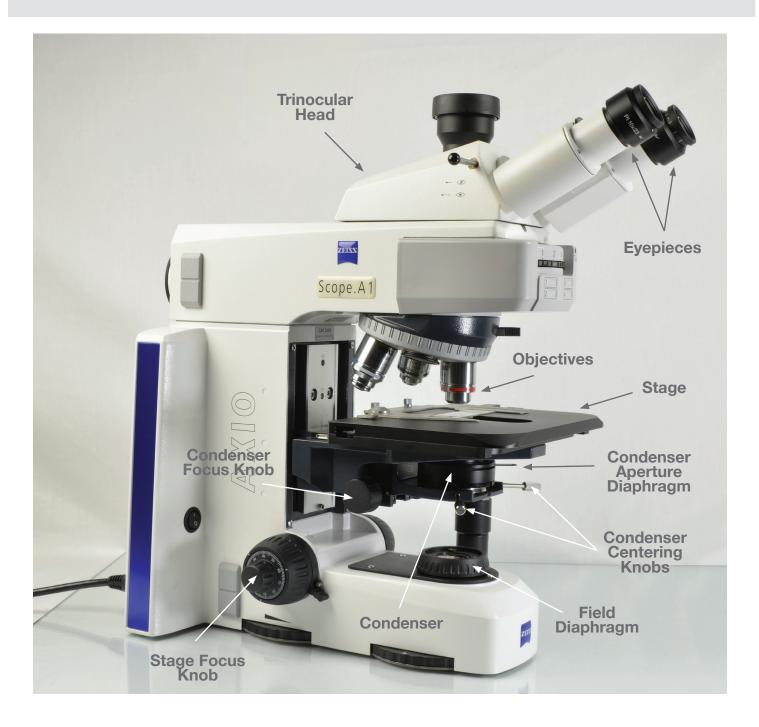
**Step 1:** Determine which objective will be used most for your detailed work. This will be the target objective for aligning the Koehler illumination.
