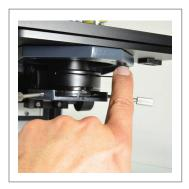
the NA setting (trading image resolution for contrast). An alternative way to set the condenser aperture is to remove the eyepiece and look down the eye tube at the back of the objective and adjust the Aperture diaphragm until approximately 90% of the area is illuminated (a setting that visually looks very near the edge of the objective but is not quite fully to the edge).
