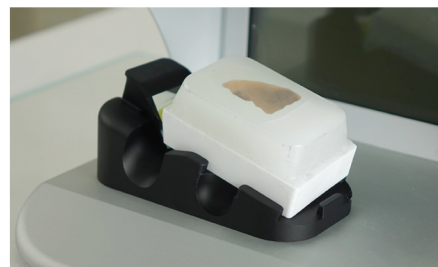
Whole Mount Sample Holder Shared Cassette / Slide Pocket With Cassette Mounted
